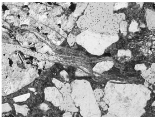
8.16 Microphotograph showing extrusion of ASR gel from impure sandstone into the adjoining cement paste (plane polarized light, view 2.8 mm \times 1.8 mm).
